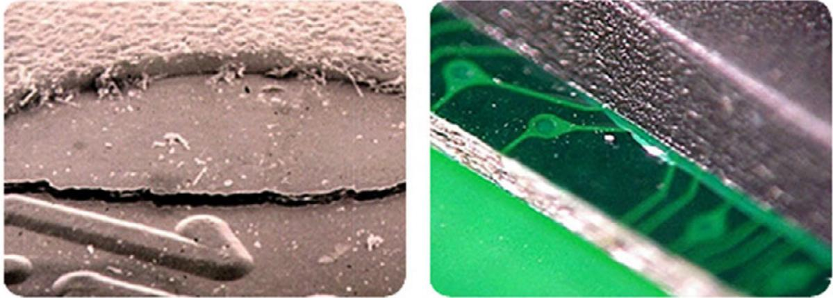
Figure 1: Component micro-cracking resulting from the absorption and rapid release of moisture.
